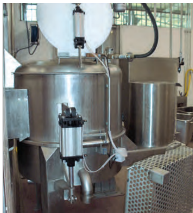
Centrifuga lavatrippe Centrifugal washing machine for tripe
