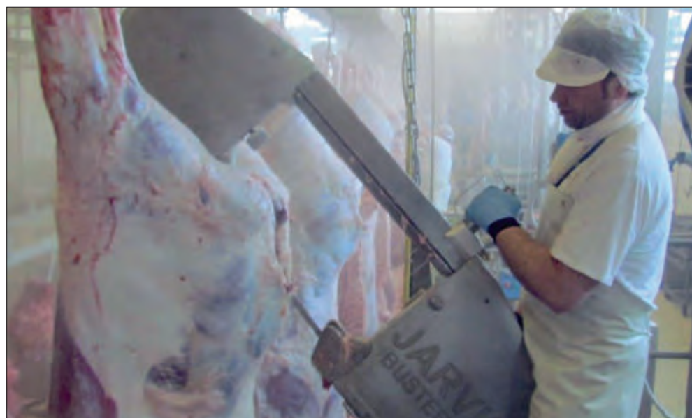
Sega mezzene bovini Cattle splitting saw in operation
