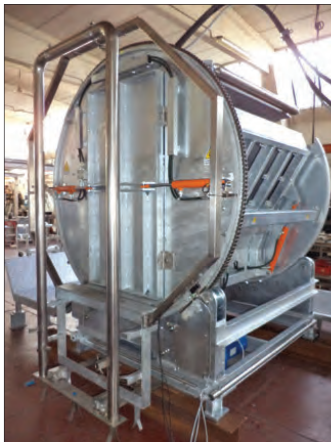
Portellone posteriore d'ingresso animale Rear inlet gate of HALAL killing box
