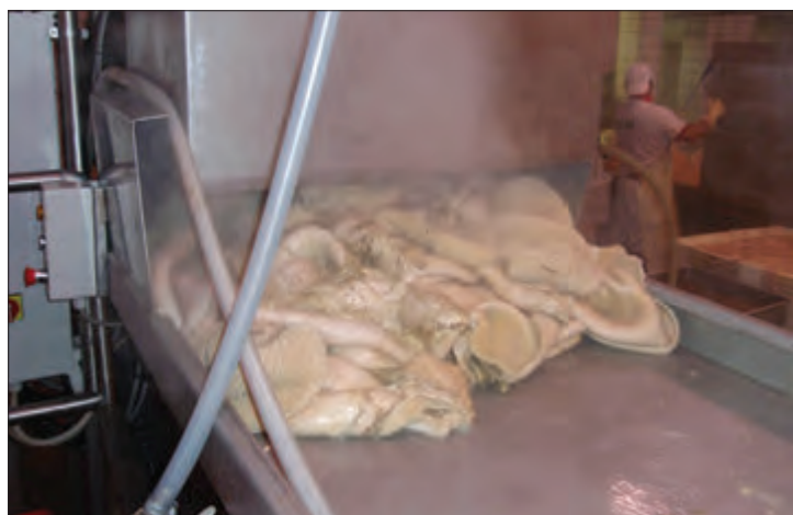
Tripe sbiancate e lavate in centrifuga Tripe washed and whitened inside centrifuging machine.
