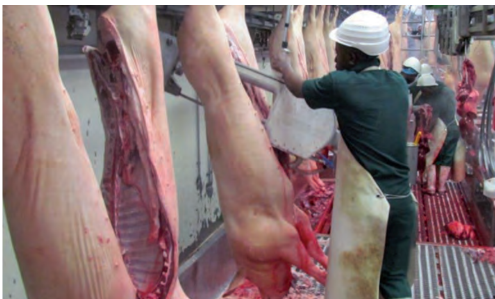
Sega mezzene suini Pig splitting saw in operation
