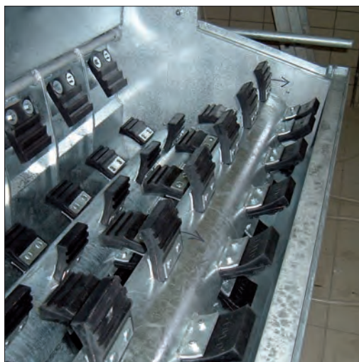
Dettaglio rulli depilscotta Details of dehairing rolls
