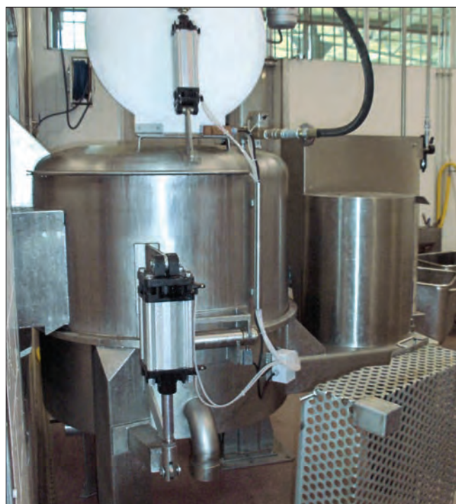
Centrifuga lavatrippe Centrifugal washing machine for tripe
