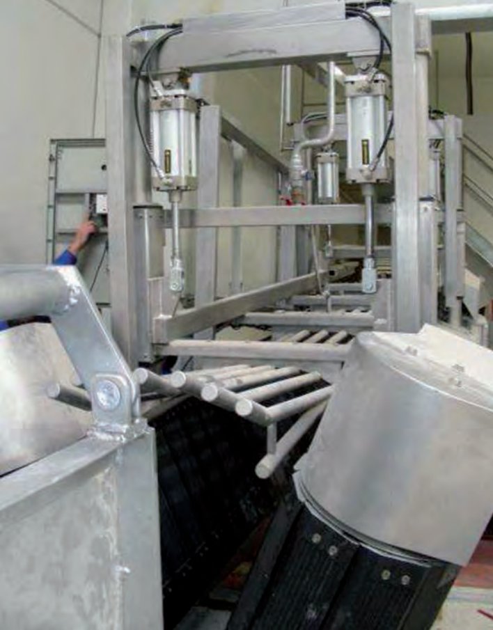
Restrainer di abbattimento suini Stunning restrainer for large production
